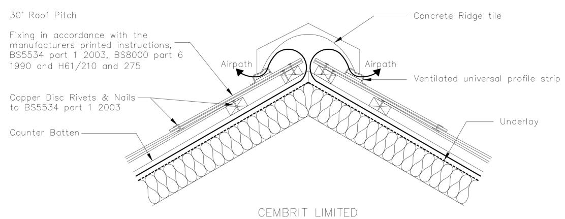
INSULATION AT RAFTER LEVEL (WARM ROOF)
